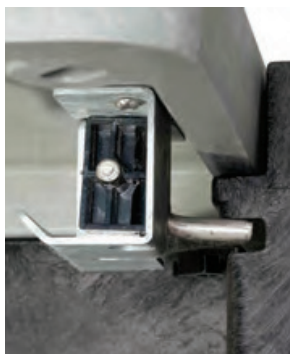
L-Bolt Security System (SHIELD Cover Shown)
